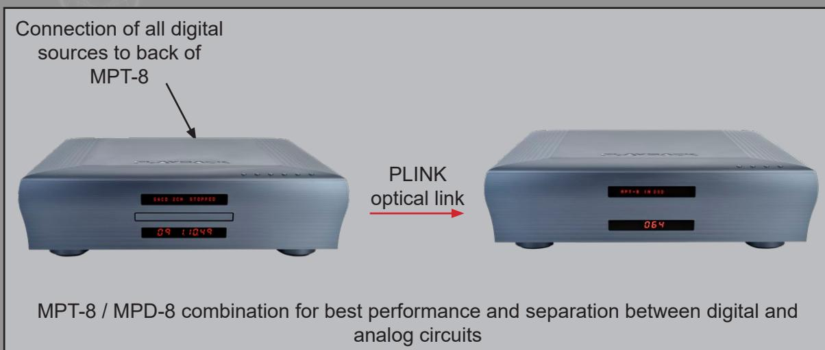
MPT-8 / MPD-8 combination for best performance and separation between digital and analog circuits
